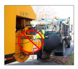
Visibility of the workers on foot is a critical component for a safe operation. In the picture on the left, the worker is between the leaf vacuum and the truck and out of the driver's sight.
